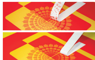
The adhesion test proves it: stencil materials adhere very well; highlight/shadow dots and fine lines stay firmly attached.
